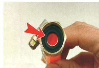
8. Check if the liquefied gas pipe gasket is missing.
