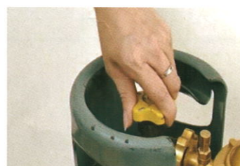
13. Turn on the liquefied gas switch.
